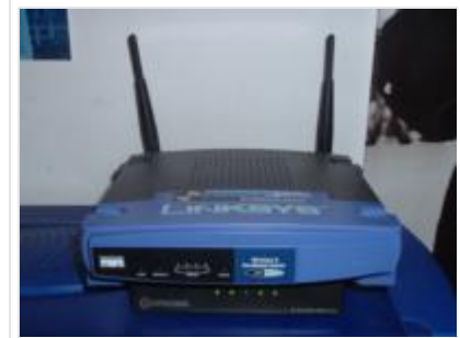
A Linksys Residential gateway with an 802.11b radio and a 4-port ethernet switch.
