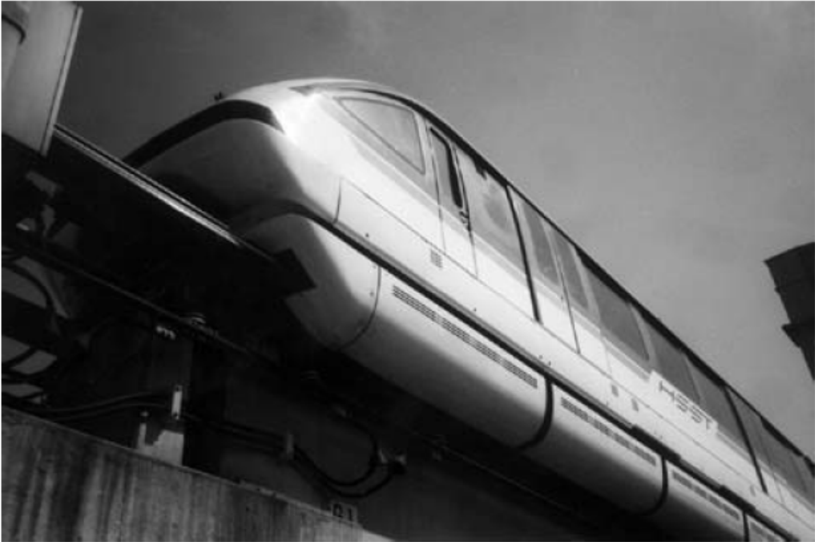
Magnetically levitated rigid body (HSST MagLev prototype vehicle, 1998, Nagoya, Japan).
